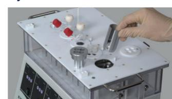
By using the test tube adapter, you can change the size and number of reaction vessel. Synthesis reaction within the scale from 0.5mL to 60mL can be implemented. Up to 20 reaction tubes can be attached.
