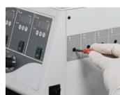
Five over heat protectors enable to set the different temperature limit for each block within the range from 60°C to 200°C. You can set the appropriate temperature depending on the type of solvent or setting temperature of the unit.
