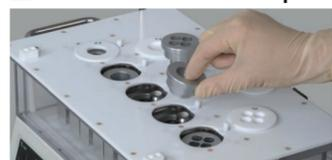
Since the reflux adapter which touches cooled reflux block, cools down the top of reaction tubes, the reaction solvent vapor can be refluxed sufficiently.
