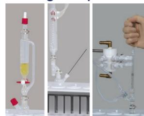
Branched reaction vessel and 3-way stopcock enable users to add sample in inactive condition or drip the sample through dripping funnel.
