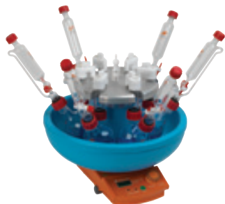
Cooled Carousel 6 Plus with 250ml flasks, Liquid Additions Dropping Funnel and Equalising Arms.
