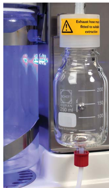
The continuously draining catch pot provides enhanced recovery of the most volatile organic solvents.
